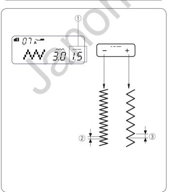
Adjusting the stitch length Press the stitch length adjustment key ----+ to change the stitch length ①.
